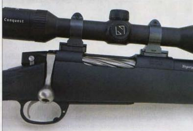
Designed by Gale McMillan, the G30 action is machined from 17-4 stainless steel, utilizes a precision-ground recoil lug that is sandwiched between the face of the receiver and the barrel shank, and accepts the same scope-mounting bases as the Rem. Model 700.
